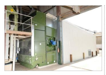
Chris Read, from Cocum Farm, Winchester, specified special side cladding to protect the drier from corrosion and reduce noise. "Our previous machine was 40 years old so obviously there are a lot of improvements on our new one. I'm particularly impressed. The greatly increased volume of air you get through makes this model far more efficient."
