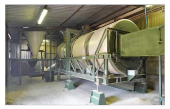
lan Baxter, of Chipmunk Equine, Salisbury, now operates an AB drier to handle wood shavings and fuels it with sawdust recovered by the dust extractor via a heat exchanger linked to a woodburner.
