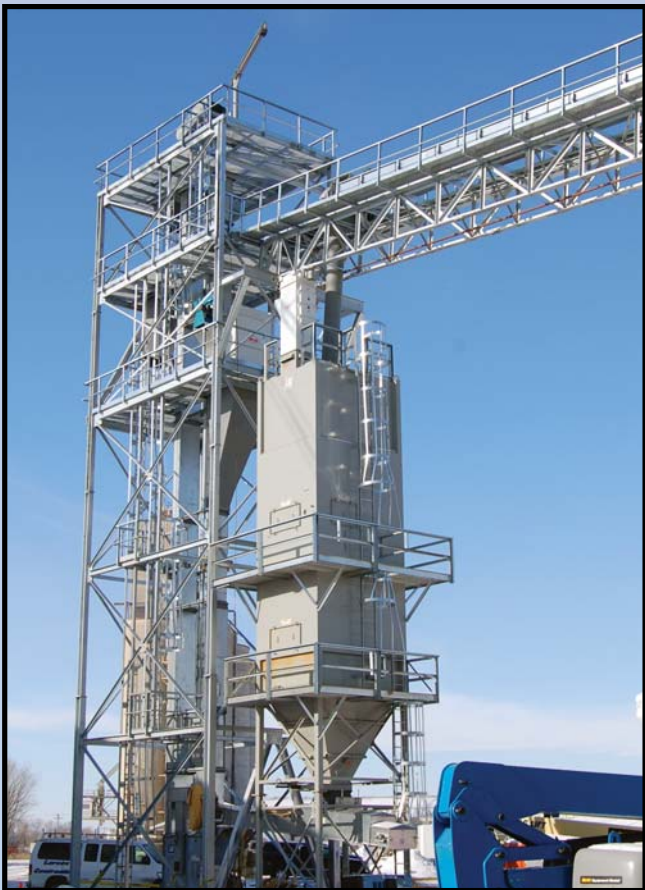
Custom catwalks and towers with top and intermediate platforms.
