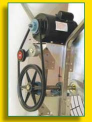
The orifice, blade, cone and motor combination optimizes the use of the motor's power curve.
