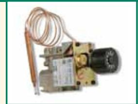
S.I.T. combines a snap-action thermostat with 100% safety cut-off valve. Modulating control provides pre-setting different BTU levels for a more constant level of heat. Brooding temperatures can be set within a range from 70° F to 115° F.
