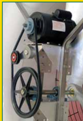
Motor mount and drive assembly utilize a rugged box frame design to increase motor life.
