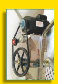
The orifice, blade, cone and motor combination optimizes the use of the motor's power curve.
