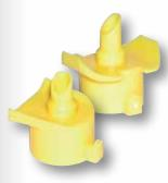
Replacement Saddles for Threaded Drinkers (VS205L / VS405L) – These saddles are a replacement for .875" square pipe (VS205L) or 1.1" square pipe (VS405L) that previously had threaded drinkers. The stems are slightly larger than the standard glued saddles so they can be glued into the existing threaded hole. These saddles accept any of our standard J-Lock Drinkers.
