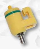
Replacement Drinker for Clark System (VR150C) This is a standard Val Drinker with a slightly modified flow pin to fit in the Clark saddle. The Clark saddle does not have the necessary clearance for the "feet" on the bottom of the Val flow pin, thus this drinker has a straight flow pin with no feet. Using this drinker to replace the Clark J-Lock, there is no need to replace the pipe, suspension or winching hardware.
