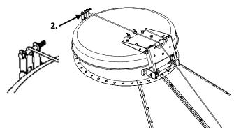
3. Guide the Cord over the bin roof (as pictured above) and use the Self- Drilling Screws to attach the Cord Retainer to the edge of the bin roof (as pictured below). 2 large holes on the Cord Re tainer are provided to allow the bin bolts to pass through. (as pictured below)
