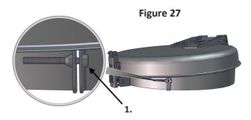
2. Wrap end of the Cord around the bolt and tie se curely. KNOT MUST BE TIGHT TO SECURE CORD. (as pictured below)
