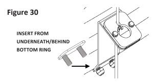
5. Slip 2 Cord Locking Collars onto the Cord. To locate the proper placement, open the lid completely and adjust the Cord Locking Collar to fit tight under the Cord Containment Bracket. Then Close the lid and place the second Cord Locking Collar tight under the Cord Containment Bracket.
