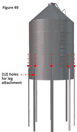
This example shows (1) leg missing to detail holes and other legs attached with red arrows to detail placement of legs continuing around bin ring.
