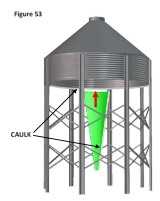
Caulk on inside Bottom Hopper Sheet along both sides of horizontal holes.
