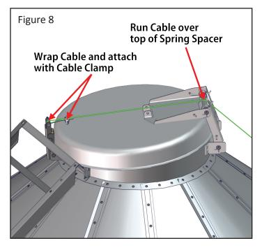
8. Wrap end of the Cable around the 500652 bolt on the Lid Latch and secure using the VC354 Cable Clamp, as shown in Figure 8 and overviewed in Figure 9.
