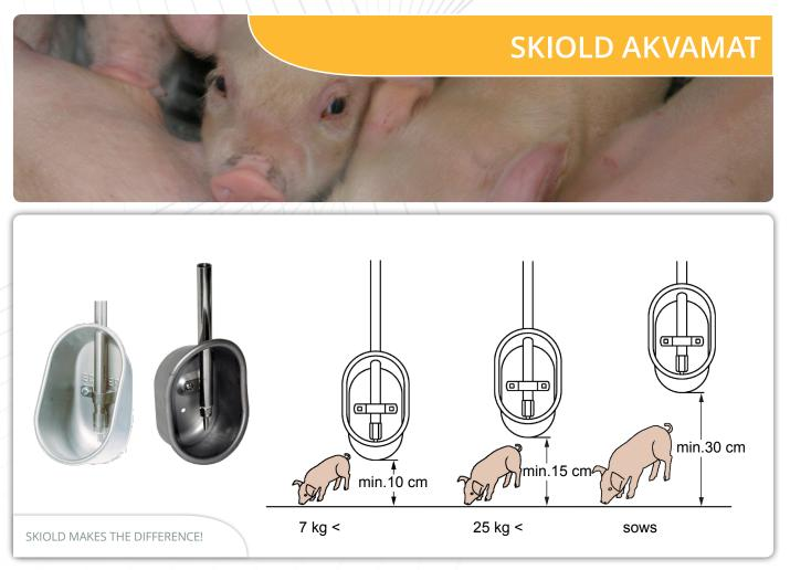
SKIOLD AKVAMAT is made from stainless steel and is available in 3 different sizes, suitable for Weaners as well as Porkers. The mounting height is adjusted to suit the size of pigs in question as shown in the sketch above. SKIOLD AKVAMAT can serve up to 20 animals per trough.
