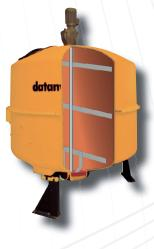
The mix-tanks are equipped with a drain, which helps to reduce remaining quantities, as well as a cleaning door with a mounted magnet to sort out any metallic foreign bodies. For storage of remaining quantities rest-tanks can be integrated with the main mixing tank. Furthermore, they will be an incorporated part of the pipe cleaning system, in which old recipes are being "pushed" out by new ones. Both the rest-tanks and mix-tanks are equipped with automatic cleaning system.
