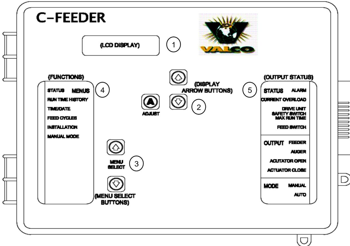
1. **LCD Display:** Shows the current information and adjustable parameters within a function.
