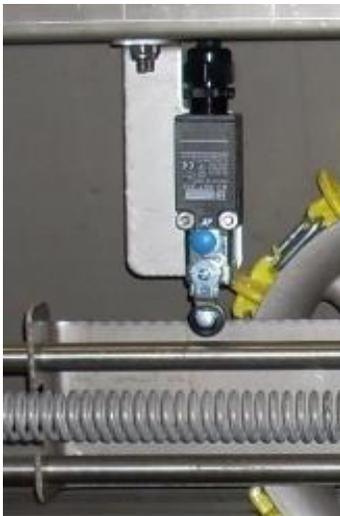
**Figure 9C** *Limit Switch Normal*
