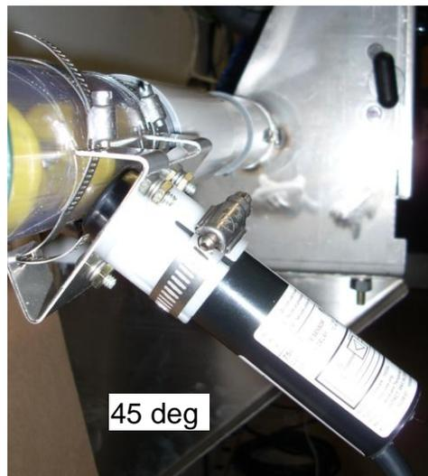
**Figure 7D** Proximity Sensor Mounting to CLEAR section of PVC
