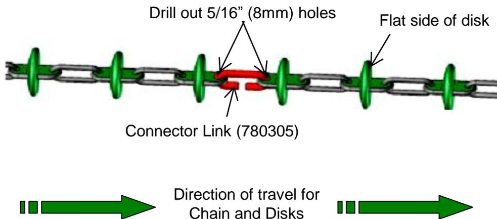
**Figure 7A** Chain and Disks with Connector Link
