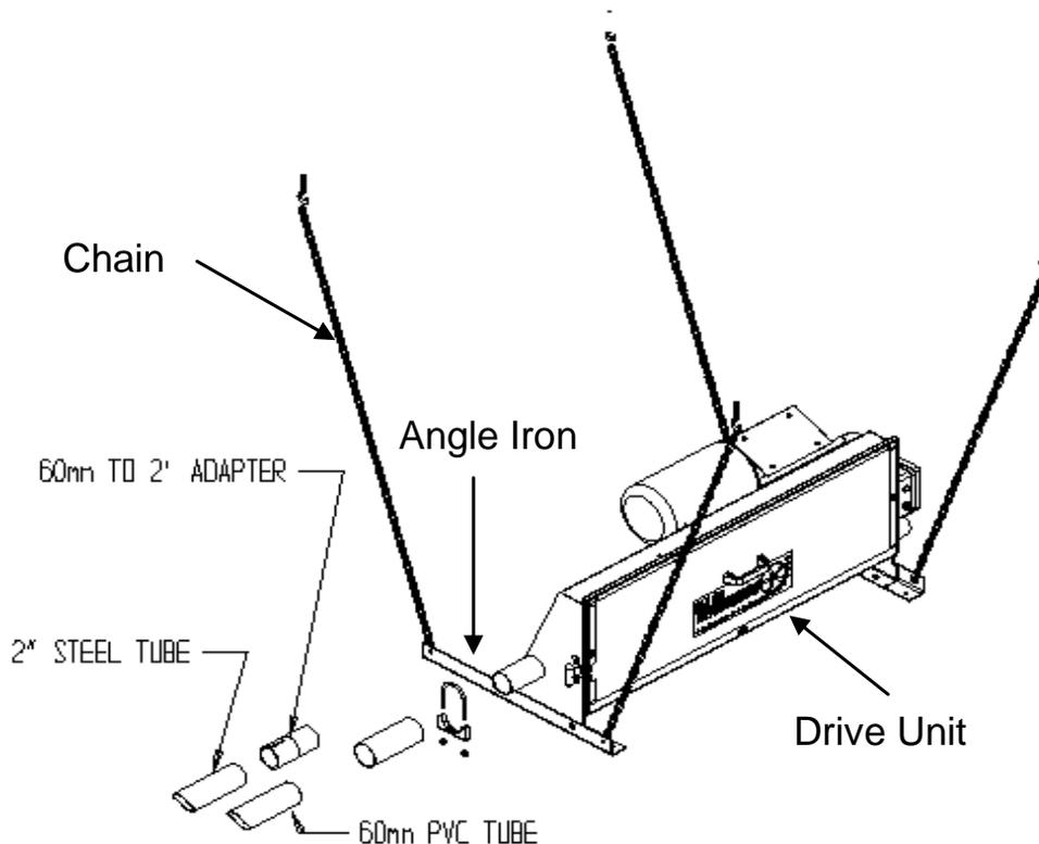
**Figure 4A** *Drive Unit Suspended Installation*
