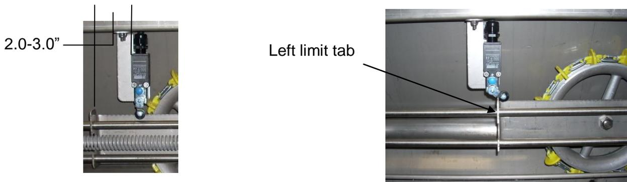
**Figure 7C** *Limit Switch Adjustment*
