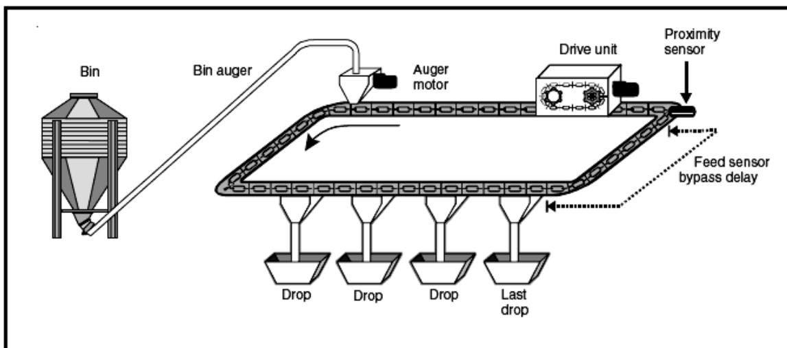
**In Continuous Mode:** A proximity sensor must be located in the tube of the last feeder drop.
