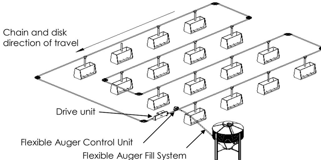
**Figure 6A** *Typical Fill System Installation*
