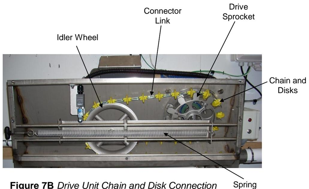
**Figure 7B Drive Unit Chain and Disk Connection**
