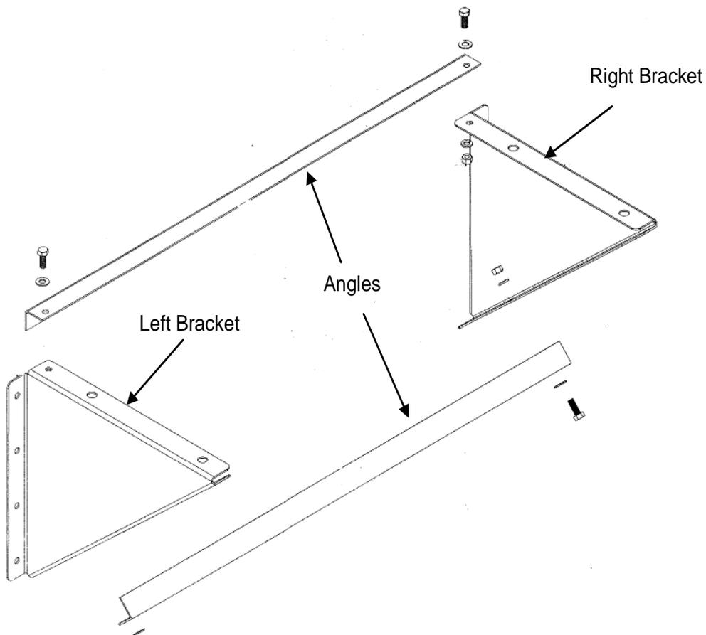
**Figure 4B** Drive Unit Wall Mount Installation
