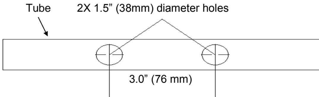
**Figure 6A** *Outlet Holes with Carry-Over*
